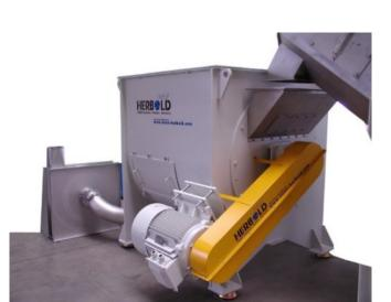
When the material enters the dryer it is accelerated with high speed. Contaminated particles and water escape through the screen perforation. The polygonal screen cage causes a turn over of the material, which leads to a better cleaning and drying result. Together with the fines the spun-off water exits the dryer through the lower discharge port.
