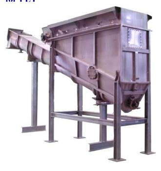
In tanks for recovery of sink fractions (specific gravity g/cm³), the material discharge is handled by oversized discharge screws.
