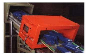
All various types of metals such as stainless steel, or copper are detectable. These types of metal cannot be identified through magnet detection but only through inductive detection.
