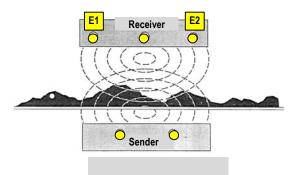
Any metallic contamination passing through this field alters the energy field. The detected unbalance in the field is analysed and converted into a switching impulse.
