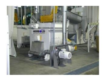
The rotor is dynamically balanced. Roller bearings outside the housing guarantee an efficiant operation of the machine. On request the rotor may be equipped with exchangeable wear plates.
