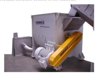
When the material enters the dryer it is accelerated with high speed. Contaminated particles and water escape through the screen perforation.
