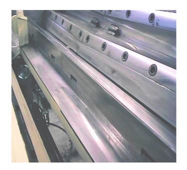
A precise and uniform rotor/stator knife cutting gap is important to ensure maximum through put rates from the granulator.
