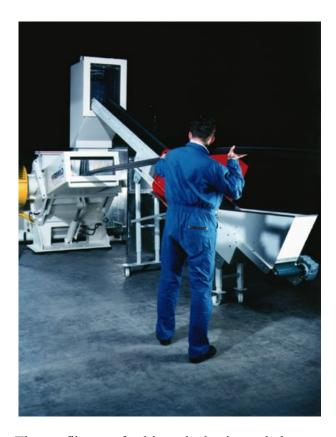
The profiles are feed into the horizontal chute, immediately grasp by the rotor and automatically pulled-in.
