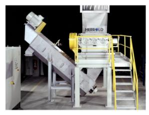
The friction washer is mounted on a zinc-coated frame in inclined position. Drive is provided by a three-phase motor and an overdimensioned V-belt drive.
