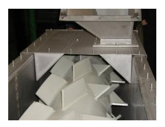
The rotor is made of a thick walled steel pipe with welded-in shaft journals and attached accelerators with additional supports. On request the rotor can be equiped with changeable paddles. The rotor is balanced in accordance to compulsory standards and guarantees an efficient operation.
